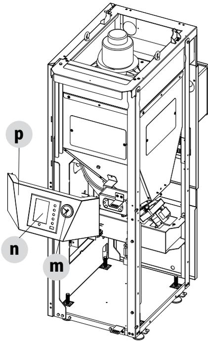
PANNEAU CENTRAL AVEC TABLEAU DE COMMANDES ET MANOMÈTRE
