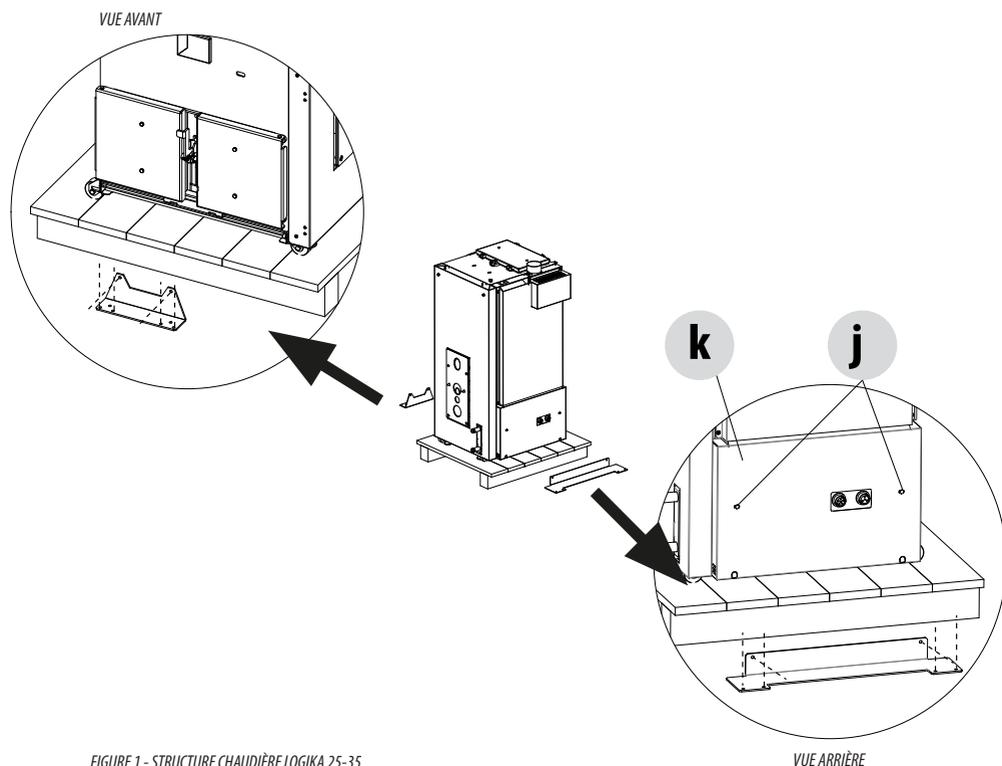
FIGURE 1 - STRUCTURE CHAUDIÈRE LOGIKA 25-35
