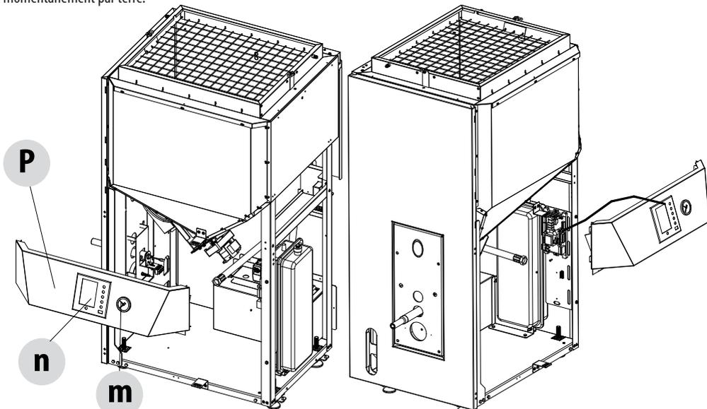
PANNEAU CENTRAL AVEC TABLEAU DE COMMANDE ET MANOMÈTRE
